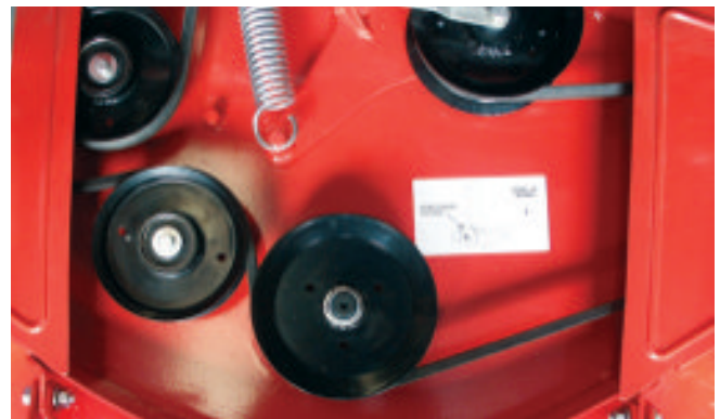
Self Tensioning Belt Blade Spindles. 20mm Shaft
