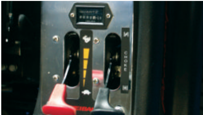
Easy Reach Control Panel. Hour Meter. PTO Switch. Throttle & Choke
