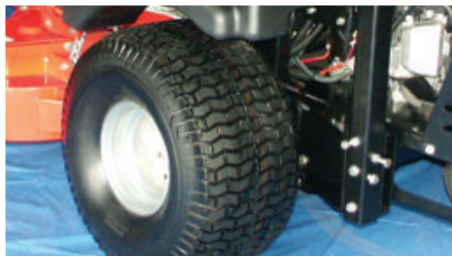
Turf-Saver. 20x10.00x8 Rear Wheel and Tyre
