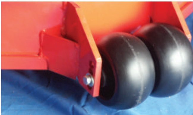
Adjustable Anti-scalp Wheels. 4 Front 2 Rear
